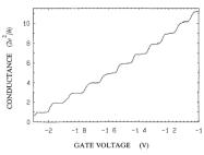
QPC conductance is quantized by steps of  $2e^2/h$
